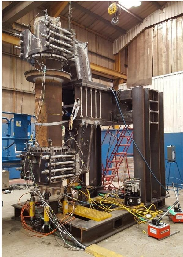
Figure 3: In-house strength and cyclic testing to validate FEA models.
