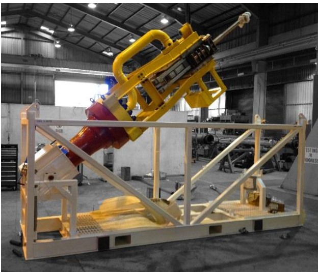
Figure 3: Left – In-house system integration test of complete Well-Stimulation System. Right – FEA model of shipping and handling basket also engineered and manufactured by Neptune.
