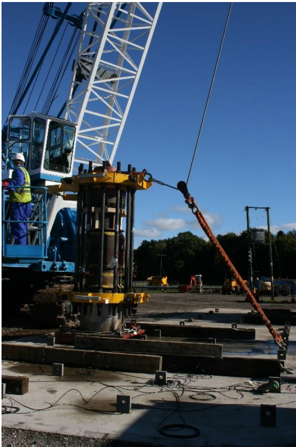
Figure 2: In-house bend tests and tension system calibration of Subsea Clamp System (using strain gauges) to validate FEA models. Excellent correlations achieved.
