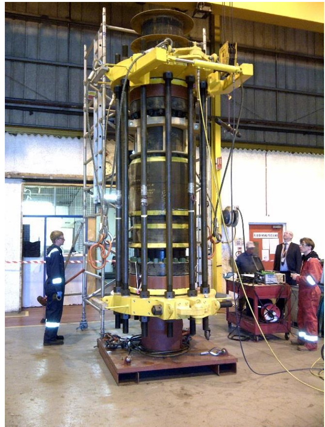
Figure 2: In-house bend tests and tension system calibration of Subsea Clamp System (using strain gauges) to validate FEA models. Excellent correlations achieved.
