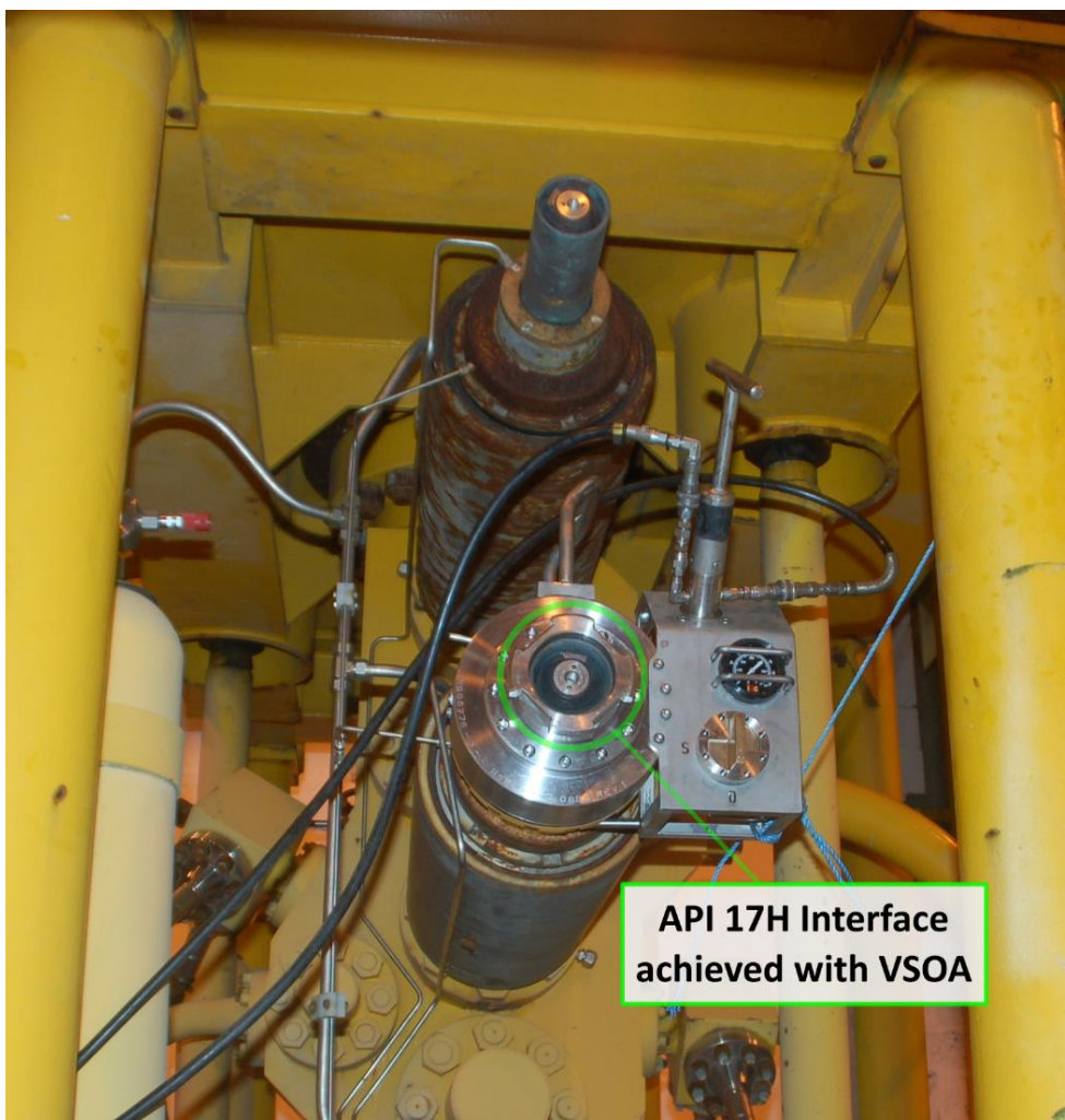
Figure 3: VSOA installed on XT valve stem, providing API 17H interface for valve override.
