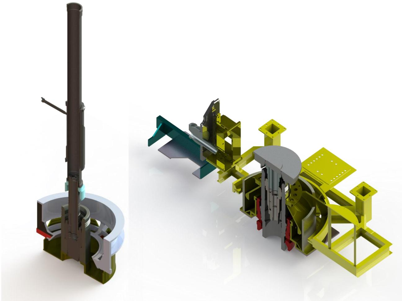
Figure 1: CAD models of wellhead, tubing hanger and tubing hanger orientation joint components, constructed for the CAD-based tolerance analysis.
